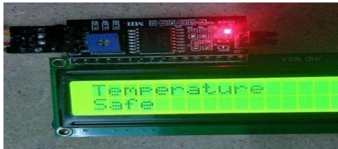
Figure 8: Displaying that Temperature is Safe in LCD
