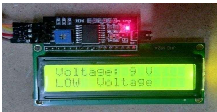
Figure 10: Displaying that Voltage Level and Condition of Voltage Level in LCD
