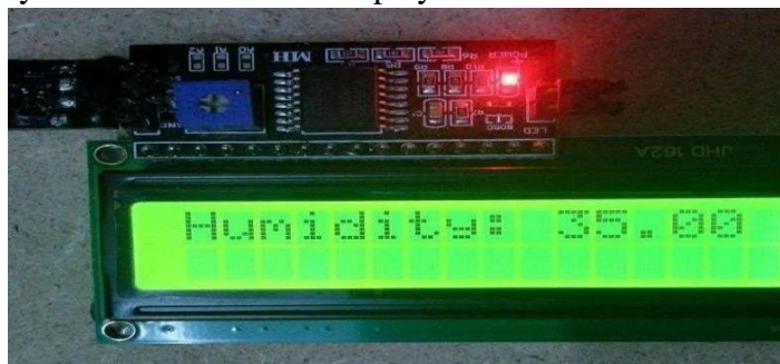
Figure 6: Displaying Humidity Value in LCD
